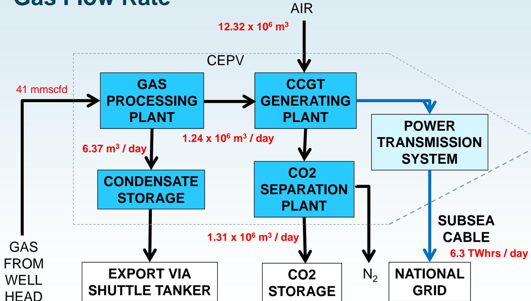
Process flow of gas to exhaust to exhaust and electrical power generation.
