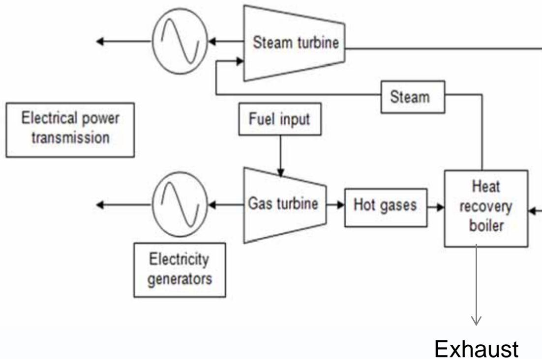
High efficiency through waste heat recovery.
